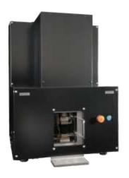
Thermal conductivity measurement methods are broadly classified into the "steady-state method" and the "non-steady-state method. The "steady-state method" measures thermal conductivity by applying a steady temperature gradient to the sample. This method is characterized by its ability to directly determine "thermal conductivity" and to measure even samples with low thermal conductivity.
